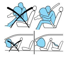
All occupants of the vehicle, including the driver, should always properly wear their safety belts, even when an air bag supplemental restraint system (SRS) is provided.
